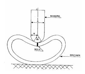
The reverse bend test shall be carried out with a mandrel. Radius (R) and width (A) of mandrel shall be calculated for any combination of diameter, wall thickness and grade with the formula.
